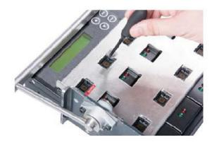
> After insert all cards into the duplicator. Pull and press the silver handle from top side to down and make sure the module fixed well.
