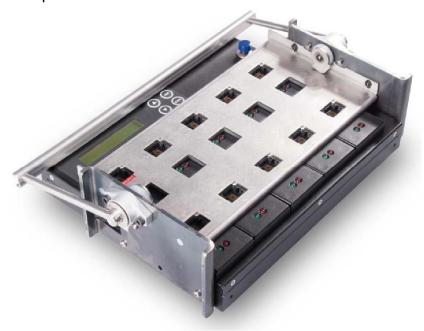
> Use the vacuum sucking pen to hold one eMMC card. Insert the card into the port. Insert all eMMC cards for tasks one by one.
